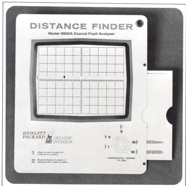
Fig. 8. This range calculating slide rule has a conversion chart for percent reflection versus worst-case return loss on the reverse side
