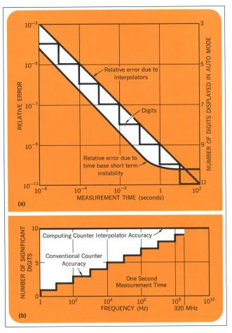
**Fig. 4(a).** Computing counter interpolator and time-base accuracy. **(b)** Computing counter interpolator accuracy compared with  $\pm 1$  count uncertainty of conventional frequency counter for one-second measurement time.
