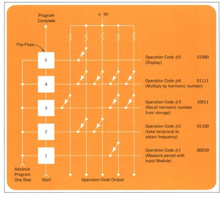
computing counter are all of the hard-wired read-only type, some made up of diode matrices (see Fig. 2) and others made up of gating networks. In addition to
