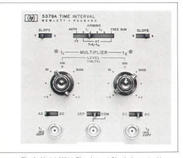
**Fig. 3.** Model 5379A Time-Interval Plug-in is used with the computing counter to measure time intervals with  $\pm 1$  ns accuracy and  $\pm 0.1$  ns resolution. Intervals down to zero can be measured, and if the stop pulse ( $t_2$  input) occurs before the start pulse ( $t_1$  input) the display will have a minus sign.
