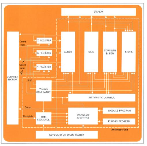
circuit. The arithmetic unit of the computing counter uses more than 400 digital IC packages which contain more than 1000 gates and flip-flops made up of more than 10,000 transistors.
