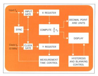
**Fig. 3.** Computing integrated circuits divide the number of input cycles (X) by the number of clock periods (Y) and multiply by  $f_Y = 10^7$  to find the unknown frequency  $f_x$ . Other IC's determine the measurement units, position the decimal point, blank insignificant digits, and apply hysteresis to prevent display jitter.
