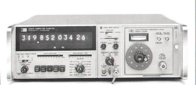
Fig. 1. Model 5360A Computing Counter is orders of magnitude more powerful than earlier counters. It measures CW or pulsed carrier frequencies between 0.01 Hz and 320 MHz to as many as 11 significant digits. Frequency-converter plug-ins extend its range to 18 GHz. It measures period (and time interval with another plug-in) with 1 ns accuracy and 0.1 ns resolution.
