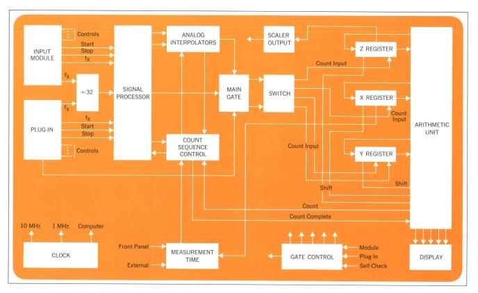
**Fig. 1.** Analog interpolators in the Model 5360A Computing Counter reduce the  $\pm 1$  count uncertainty by a factor of 1000. The arithmetic unit provides the computational capability needed to make use of interpolation. When the counter is counting, the X, Y, and Z registers act as decade counting assemblies.
