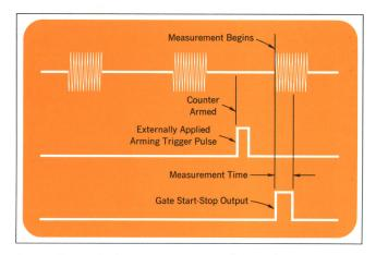
**Fig. 2.** External triggers or gates can be applied to the computing counter to make it measure the frequency of any part of a burst of a carrier signal. The measurement starts with the next input cycle after the leading edge of the trigger or gate. The counter will also measure the frequency of a single burst without external gates; it arms itself, then starts counting with the first input cycle.
