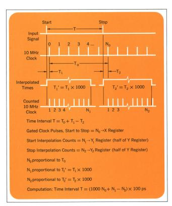
**Fig. 2.** Time interval is the basic measurement of the computing counter. The small times  $T_1$  and  $T_2$  represent the phase difference between the input start/stop signal and the internal clock. In an ordinary counter, which counts only  $T_0$ , these times account for the  $\pm 1$  count uncertainty. In the computing counter, the analog interpolators stretch  $T_1$  and  $T_2$  1000 times, giving the counter a time-interval resolution of 0.1 ns although its clock rate is only 10 MHz.
