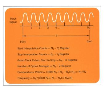
**Fig. 3.** For period and frequency measurements the computing counter's measurement cycle is synchronized with the input signal. The selected measurement time is actually a minimum value; the actual time is an integral number of input periods. Besides measuring  $T_{o}$ ,  $T_{1}$ , and  $T_{2}$  as for time interval, the counter counts the input periods  $N_{x}$  and then computes period or frequency.
