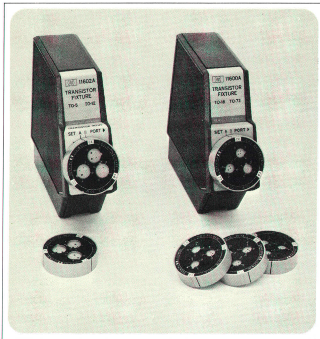
Fig. 2. Transistor fixtures have snap-on pin identifying masks which tell where to insert the transistor leads. The fixtures swallow leads up to 1.5 inches long and take them completely out of the measurement.
