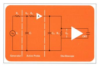
Fig. 5. Equivalent circuit of a typical active probe.
