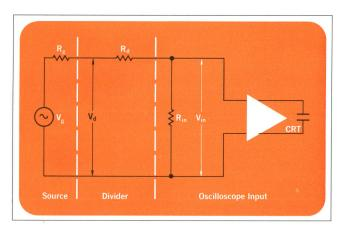
Fig. 3. Division ratio in a typical resistive divider probe is determined by  $R_{\rm d}$ ,  $R_{\rm g}$  and  $R_{\rm in}$ .
