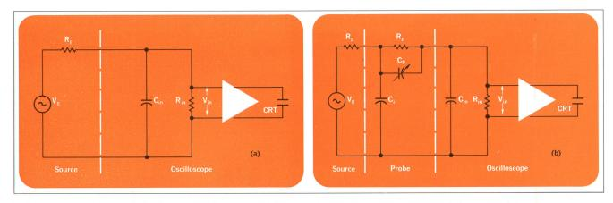
Fig. 1. Typical oscilloscope input (a) is a low pass filter whose characteristics depend upon source resistance and input capacitance. Addition of a probe (b) enables input capacitance to be reduced and source resistance to be increased thus improving high-frequency performance of the typical input.
