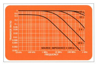
Fig. 6. Transfer ratio plots of an active probe with an input impedance of 100 k ohms and 3.5 pF input capacitance.
