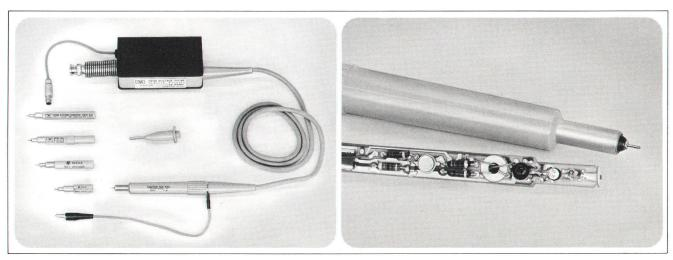
Fig. 1. Various tips (left) may be used with the HP Model 1123A Voltage Probe to increase dynamic range or ac couple the probe. The spring mounting of the amplifier assembly reduces the possibility of connector damage. Fig. 2. By mounting a FET in the probe tip and using miniature components, the input capacitance is kept low.
