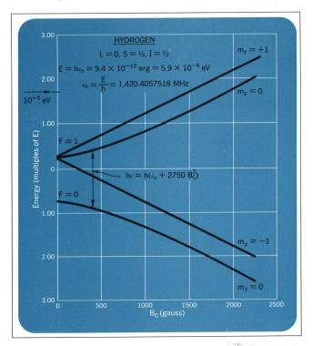
Fig. 3. In the hydrogen maser, the desired transition is from energy state F = 1,  $m_F = 0$  to energy state F = 0. The energy of this transition, and therefore the maser's operating frequency  $\nu$ , depend upon the magnetic field  $B_c$ , so maser cavities are carefully shielded to eliminate stray fields.
