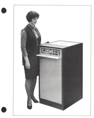
Fig. 5. The latest version of the hydrogen maser is much smaller and more rugged than previous designs. Two masers similar to this one but without cabinets will be put into orbit in a satellite to test the gravitational red shift predicted by Einstein.
