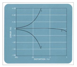
Effect of even harmonics on average-reading voltmeters (Curve 2), and on peak-reading voltmeters (Curve 1).
