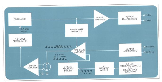
Fig. 3. Precise positive and negative 9.9-volt dc references are responsible for the accuracy of the Model 745A. The rms value of the square wave produced from these two voltages is the standard to which the oscillator rms voltage is compared. Oscillator output level is corrected by the AGC signal from the full-wave demodulator.
