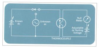
Fig. 1. Basic ac-dc thermal transfer measurement setup. By adjusting the voltages so a null is obtained for both the dc and unknown ac voltages, the rms value of the ac is equal to the known dc.
