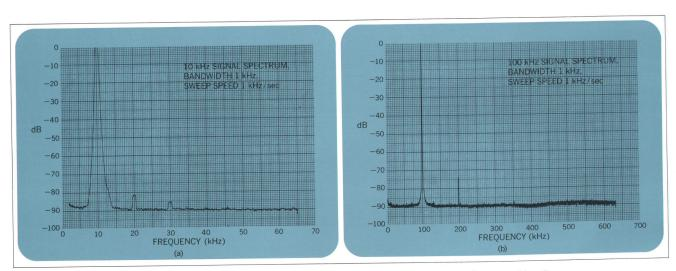
Fig. 6. Harmonic output of the Model 745A is better than 70 dB down, making it useful as a low-distortion oscillator, as well as a high-purity calibration standard.
