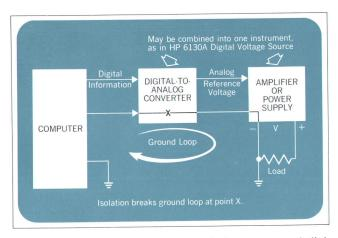
Fig. 4. Whenever a power supply is programmed digitally, there should be no connection between the ground of the digital inputs and the ground of the analog output. Without isolation, small voltage drops in the power supply leads can cause large circulating ground-loop currents. In the new digital voltage sources, isolation is provided by oscillators with transformer-coupled outputs, one for each input data bit.
