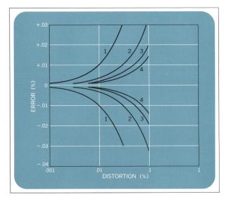
Effect of odd harmonics on average-reading voltmeters (Curves 2, 3, 4), and peak-reading voltmeters (Curve 1).
