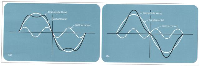
In-phase third harmonics (a) add the area of an extra half-cycle to the envelope and cause a higher than rms reading of an
