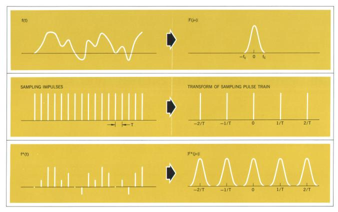
Fig. 5. Band-limited signal (top) sampled by infinite impulse train (middle) has frequency spectrum consisting of original spectrum duplicated at multiples of sampling frequency 1/T. No information about signal is lost as long as duplicate spectra do not overlap, i.e., as long as  $1/T > 2f_c$ , where  $f_c$  is highest frequency present in signal f(t).
