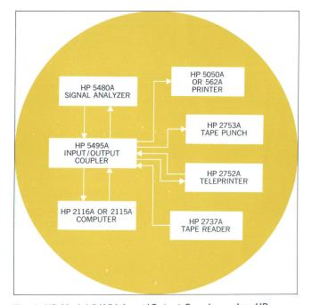
Fig. 1. HP Model 5495A Input/Output Coupler makes HP 5480A Signal Analyzer compatible with computer, printer, teleprinter, tape reader, and tape punch. Any or all peripherals can be added to system simply by plugging card/cable assemblies into back of coupler.
