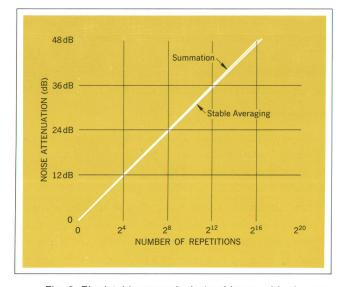
Fig. 2. The 'stable averaging' algorithm used in the new signal averager takes a few more repetitions than summation to achieve the same noise attenuation. The big advantage of stable averaging is that the display remains calibrated at all times instead of growing off-scale. The new averager also has a summation mode.
