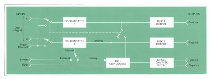
Fig. 3. Single channel analyzer block diagram.
