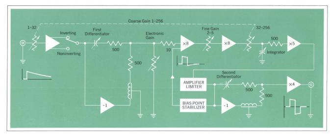
Fig. 2. Linear amplifier block diagram.
