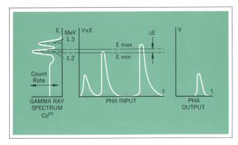
Fig. 9. When the two discriminators of the analyzer are adjusted to form a 'window,' only pulses whose level falls within the window range will produce a pulse output from the pulse height analyzer.
