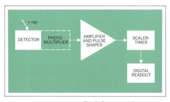
Fig. 5. Gross counting measures radiation intensity regardless of energy.
