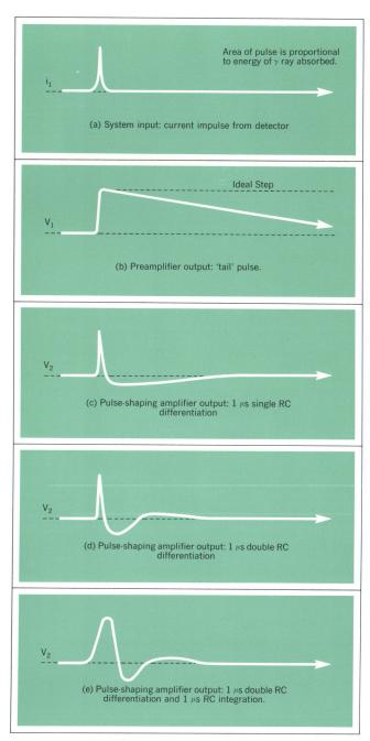
Fig. 14. Typical waveforms in signal-processing system.
