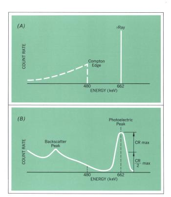
Fig. 3. Gamma spectra of Cs<sup>137</sup> gamma radiation (A) Ideal, (B) Typical in practice.
