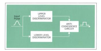
Fig. 8. With two discriminators, the system can be made to respond only to pulses whose peak value falls within a selected range.
