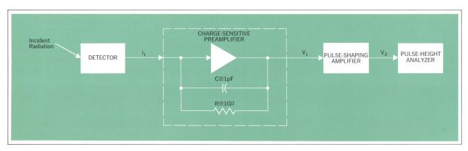
Fig. 13. Typical signal processing system.
