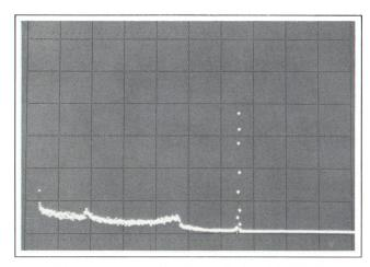
Fig. 2. Multichannel analyzer displays energy spectrum of Cs<sup>137</sup>. Solid-state detector was used, Number of pulses (vertical) is displayed as a function of energy (horizontal).
