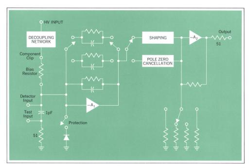
Fig. 3. Block diagram of preamplifier.
