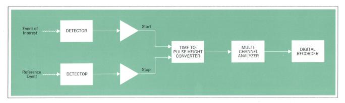
Fig. 12. Measuring arrangement to obtain a spectrum of the time-intervals between two related events.
