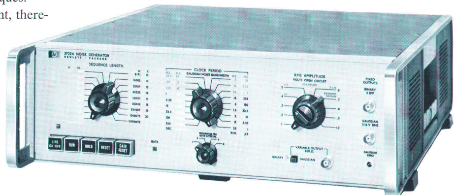
Fig. 1. A precision digital instrument, Model 3722A Noise Generator synthesizes repeated pseudo-random noise-like patterns or non-repeating random noise. Binary (two-level) and Gaussian (multi-level) outputs are generated. Amplitudes and bandwidths of outputs and lengths of pseudo-random patterns are variable.
