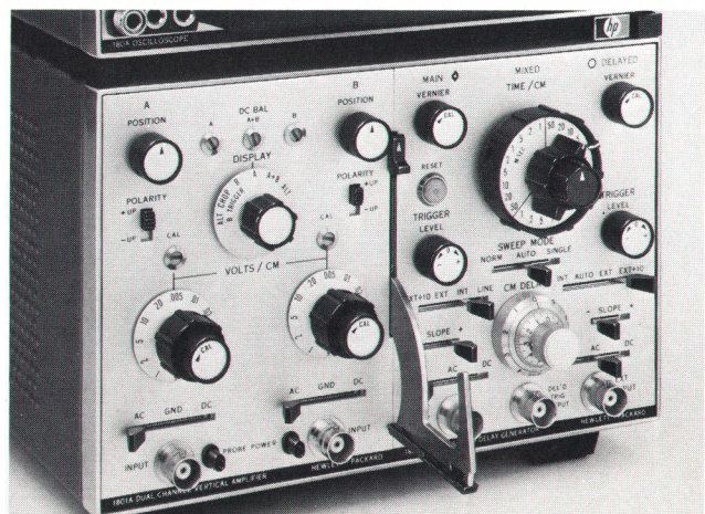
Fig. 14. Latch pulls down making it easy to remove the plug-ins.
