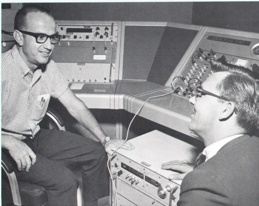
Flying clock (below counter) is compared to NBS frequency and time scales in "clock room" at Boulder Laboratories of National Bureau of Standards. Dr. James Barnes (left), Chief of Atomic Frequency and Time Standards at NBS, and -hp- engineer Lee Bodily discuss techniques of time measurement.
