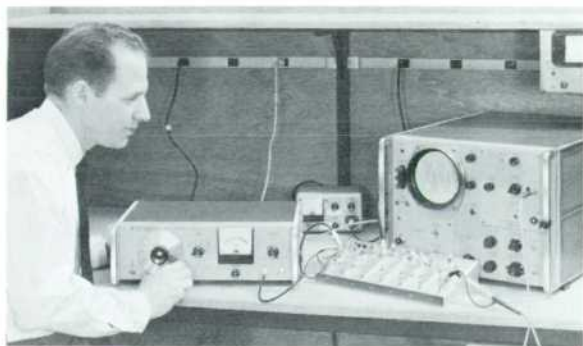
Fig. 2. Solid-state test oscillator has wide frequency range and output flexibility required by laboratory applications. Accurate attenuator and monitor meter assure well-defined output power levels. New test oscillator has frequency and amplitude stabilities of high order.
