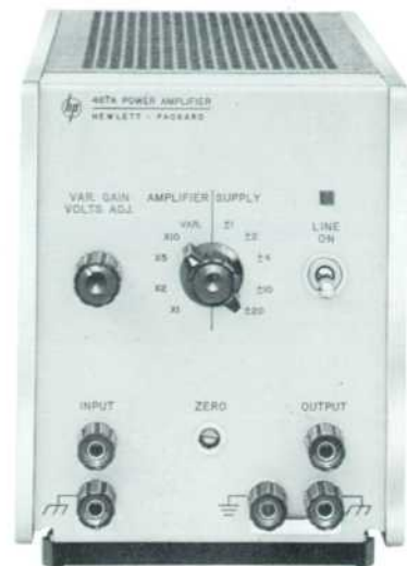
Fig. 9. Model 467A Power Amplifier has maximum output of \pm 20 V peak at 0.5 amp peak, and response that extends from dc to beyond 1 Mc/s.
