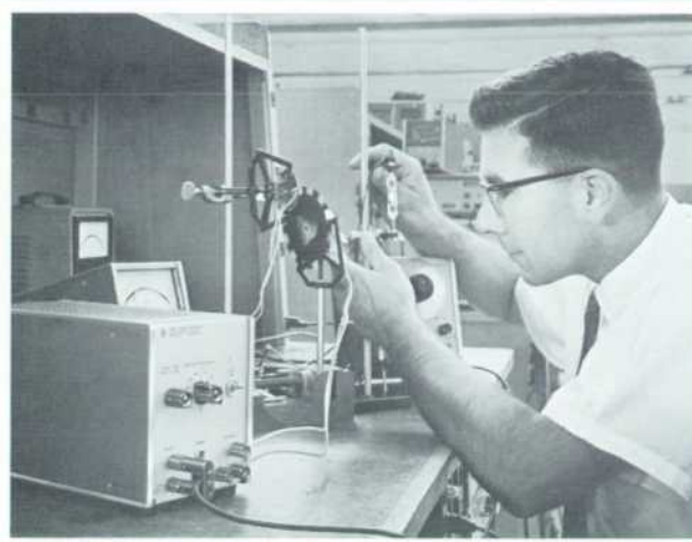
Fig. 1. New Model 467A Power Amplifier (foreground) combines dc coupling and greater than 1 Mc/s response with power capability. Here it increases output power of test oscillator for driving synchronous motor in frequency response test of photodetectors. New amplifier also serves as \pm 20\text{ V} , \frac{1}{2} -amp power supply.
