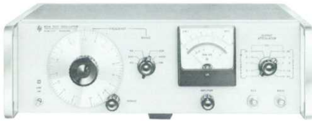
Fig. 6. New -hp- Model 651A Test Oscillator has calibrated outputs for either 50 or 600 ohms but can drive any load impedance without distortion throughout 10 c/s to 10 Mc/s frequency range. Options provide for outputs calibrated for and matched to higher impedances.
