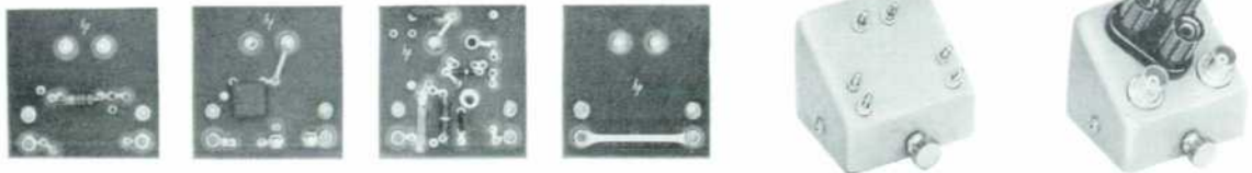
Fig. 4. Test circuit cards and holders provided with Tester. Circuits of cards are shown in other illustrations. Right-hand card permits viewing test pulse.
