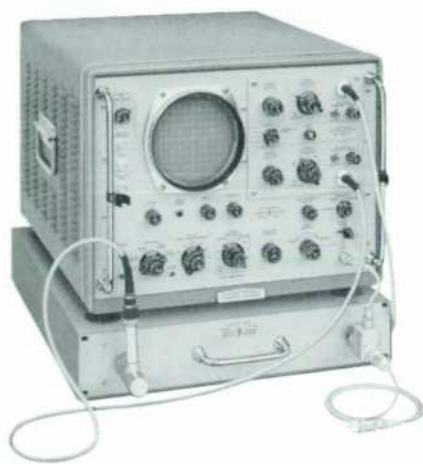
Fig. 3. -hp- 185B/187B Oscilloscope with Model 1100 Delay Line (lower unit) for use if measured circuit does not provide trigger.
