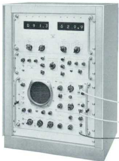
Fig. 1. Dymec Automatic Waveform Measuring System makes rapid time-interval measurements, such as switching times of high-speed transistors and diodes.
