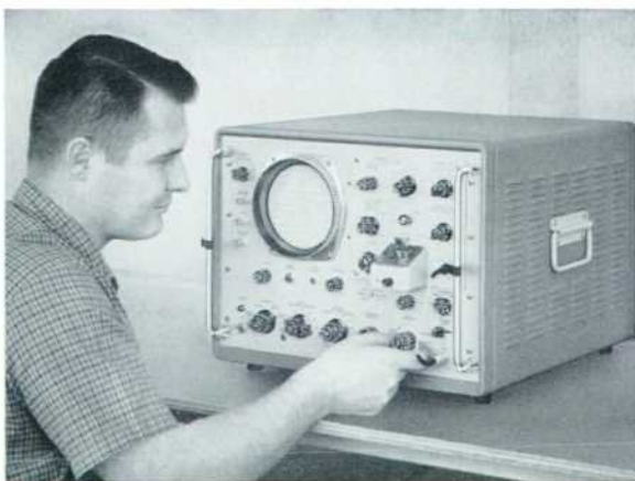
Fig. 1. New -hp- Model 186A Switching Time Tester plug-in operates with -hp- Model 185A or 185B Sampling Oscilloscope to measure rise, fall, switching, and recovery times of fast transistors, diodes, tunnel diodes. Device to be tested simply plugs into test circuit provided on holder. Tester provides fast test pulse and adjustable voltages for operating device.
