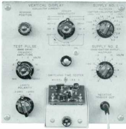
Fig. 3. Panel detail of new hp-186A Tester. Holder has test transistor plugged into test circuit on card.
