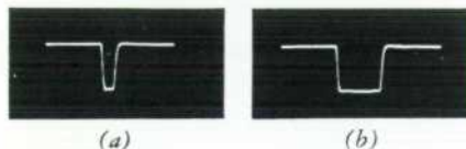
Fig. 3. Typical (a) 0.25-microsecond and (b) 1-microsecond r-f output pulses (detected). Most instruments generate pulses as short as 0.25 microsecond, although specified minimum width is 0.5 microsecond.
