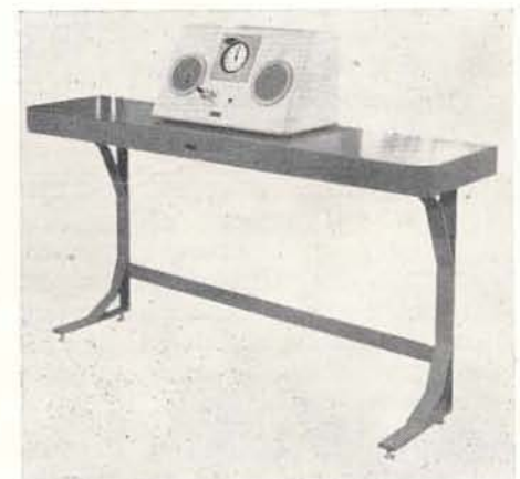
The above picture is one of 16 producer cabinets, designed for each of the 16 studios. They are equipped so that a program producer can maintain simultaneous 2-way communication with the control room by the two loudspeakers.
