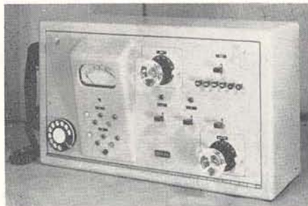
Ten tape cabinets like the one pictured above were installed in 10 tape playback machines. Facilities on this tape cabinet were such that a tape program on either of the tape machines could be selected and routed to either Master Control or recording console at the same time or to a Studio C Console.
