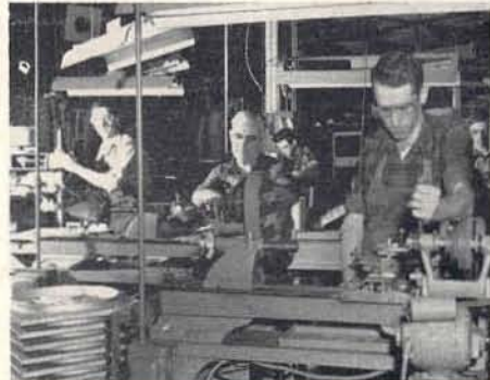
Ed. Kabrick, Bill Weed, Sr., and Frank Bruening operating different pieces of Machine Shop equipment. Ed is operating a radial drill, drilling base castings for the CB-11 turntables. Bill is machining parts to close tolerances to be used in transmitter assembly, and Frank is machining parts to be used in the tooling of fixtures and dies.
