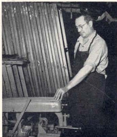
The power saw is being run by Harry Milbert. He is cutting material that will be fabricated into transmission line brackets.
