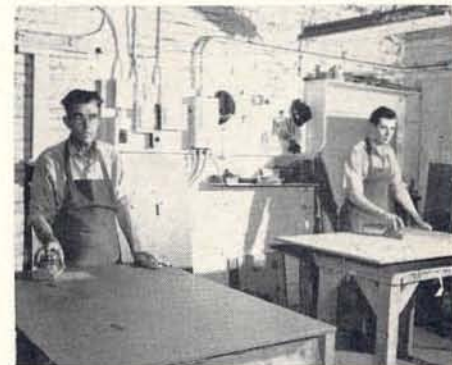
Bill Hopper and Jim Griffith complete sanding operation before finish coat is applied in spray booth.
