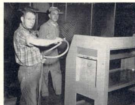
Sterling Johnson and Bob Nixon have just completed spraying the finish coat on a Gates sound effect console.
