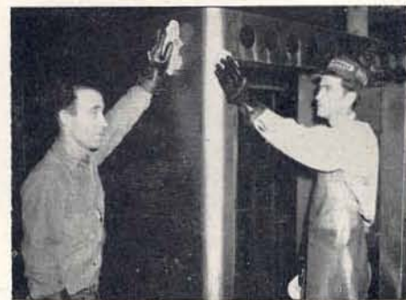
Harold Bennett and Wayne Shores are busy cleaning a BC-1F cabinet before it goes into the paint room. All units must be cleaned and degreased in an Oakite solution before the primer coat is applied and before the finish coat is sprayed.
