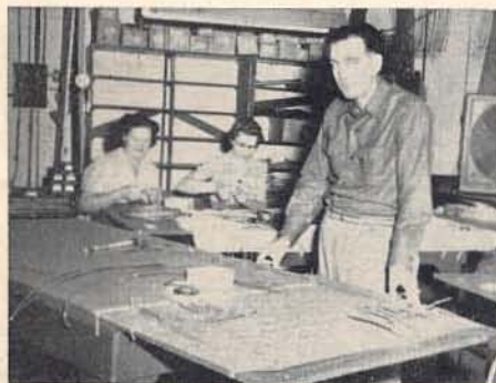
Assistant Foreman Kenny French, in charge of the cable section, is shown starting the layout of a new cable. In the background Lavina Fahey and Gertrude Gish are busy numbering and putting lugs on wires.
