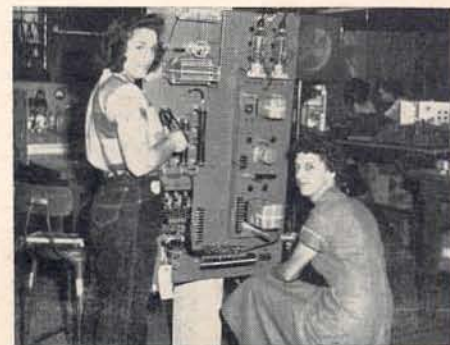
Lurene Winkler and Luellen Pryor are assembling controls and modulator panels for 250 GY Transmitters.
