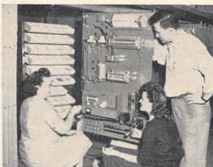
Assistant Foreman Clarence Moritz instructs while Mary Ellen Rupp and Helen Metzger assemble R. F. section for 250 GY Transmitter. In the background is one of our new parts bins for small hardware. The detachable bins can be lifted from the rack and attached to the bench rack at each assembly point.
