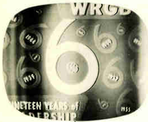
Tele-Clue D-239 and 240 Open C-209 in Vertical Blanking Circuit
