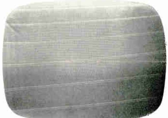
TELE-CLUE M-221: The intermittently blank screen shown above was particularly difficult to locate since its occurrence was unpredictable and only lasted a few seconds when it did occur. Both sound and picture would disappear momentarily and then reappear and operate normally sometimes for hours. The defective component was an intermittently open capacitor, C379A, in a General Electric Model 17T1. When capacitor C379A, shown in Figs. 2 and 3, "opened," the horizontal waveform which has considerable amplitude (about 200 V peak-to-peak) was fed from the plate of V13B through R369, R367, R273 and C351 to pin 4 of V11. The amplified horizontal waveform was then passed through R353, C353 and C354 to pin 1 of V11. At this point, due to the amplitude of the waveform, a high negative AGC voltage was developed which cut off the RF and IF amplifier tubes. This resulted in complete loss of both sound and picture.
