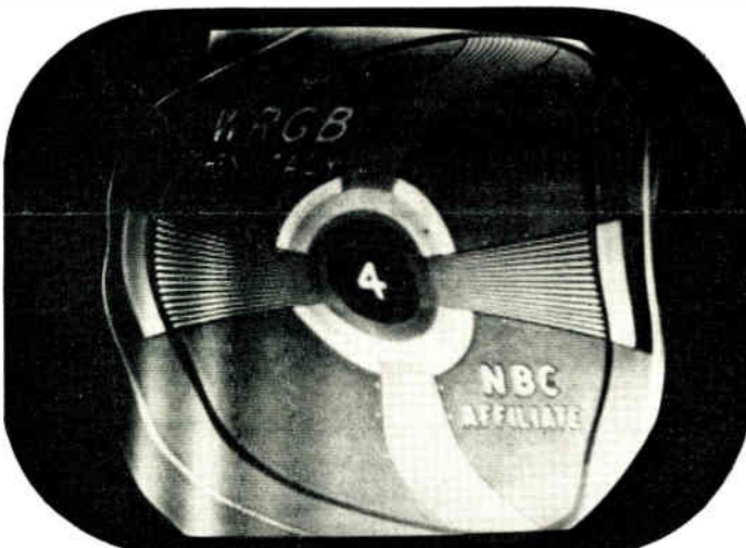
Tele-Clue No. F103. This photo indicates a defective component which reduces the output B+ voltage. This reduced B+ voltage will affect both horizontal and vertical sweep and will also give reduced picture brilliance. The ripple and shadow through the picture is due to inadequate filtering of the "B" supply. This was caused by an open C452 in Figure 2.
