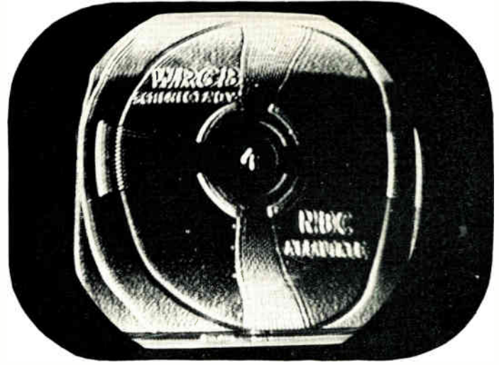
Tele-Clue No. M102. This condition is typical when a component fails in the AGC circuit. It may result in the contrast control having little or no effect on the picture. If the contrast control has little control, it may be due to leakage in one of the capacitors such as a C261 or C251. Since the impedance of the circuit is high, leakage in the order of 1 megohm or less may cause trouble. A completely inoperative control may be the result of a shorted capacitor or a ground in the AGC system. This was caused by a shorted C251 in Figure 2, however, a short in C261 or an open in L258 may result in a similar condition.
