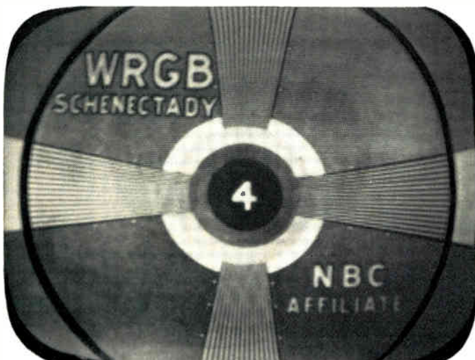
Tele-Clue No. F-110. This photograph was taken of the same receiver with the line voltage increased to 130 volts. No other adjustments were made. The width and height have increased and the black portions of the test pattern are darker. The definition of the vertical wedges is reduced near the center of the picture which could have been corrected by adjusting the focus control.
