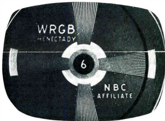
TELE-CLUE G-167: Loss of brightness may be caused by a reduction in the strength of the ion-trap magnet. The above picture indicates the maximum brightness that could be obtained with an ion-trap magnet which had lost some of its magnetism. A similar condition may be caused by an incorrect adjustment of the ion-trap magnet or incorrect voltages on the picture tube.
