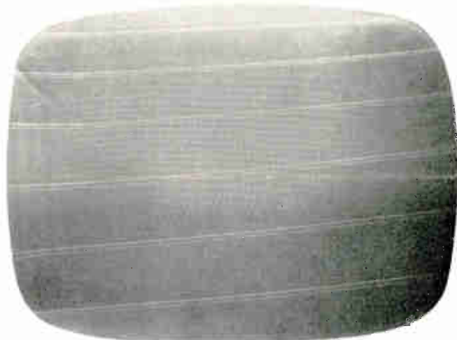
TELE-CLUE M-221: The intermittently blank screen shown above was particularly difficult to locate since its occurrence was unpredictable and only lasted a few seconds when it did occur. Both sound and picture would disappear momentarily and then reappear and operate normally sometimes for hours. The defective component was an intermittently open capacitor, C379A, in a General Electric Model 17T1. When capacitor C379A, shown in Figs. 2 and 3, "opened," the horizontal waveform which has considerable amplitude (about 200 V peak-to-peak) was fed from the plate of V13B through R369, R367, R273 and C351 to pin 4 of V11. The amplified horizontal waveform was then passed through R353, C353 and C354 to pin 1 of V11. At this point, due to the amplitude of the waveform, a high negative AGC voltage was developed which cut off the RF and IF amplifier tubes. This resulted in complete loss of both sound and picture.
