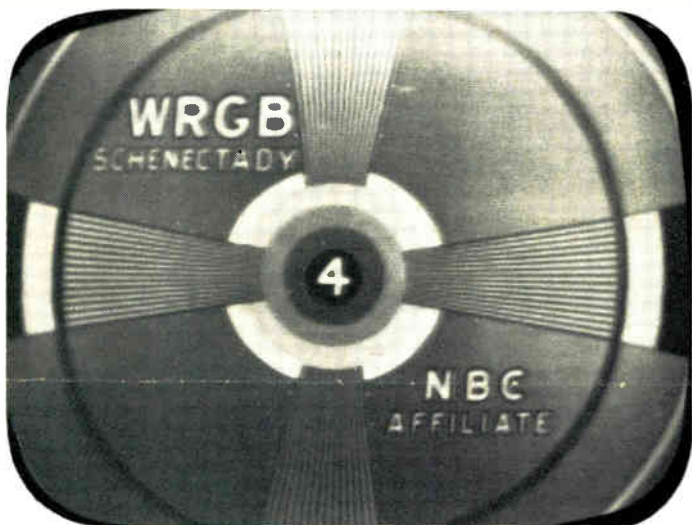
Tele-Clue No. F-109. Line voltage variations will affect the over-all operation of a TV receiver. The height, width and focus are all affected as can be seen by comparing the four Tele-Clues shown on this page. The above photograph was taken after the TV receiver was adjusted for proper operation at a line voltage of 120 volts.
