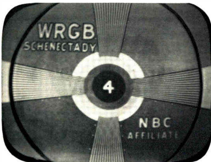
Tele-Clue No. F-110. This photograph was taken of the same receiver with the line voltage increased to 130 volts. No other adjustments were made. The width and height have increased and the black portions of the test pattern are darker. The definition of the vertical wedges is reduced near the center of the picture which could have been corrected by adjusting the focus control.
