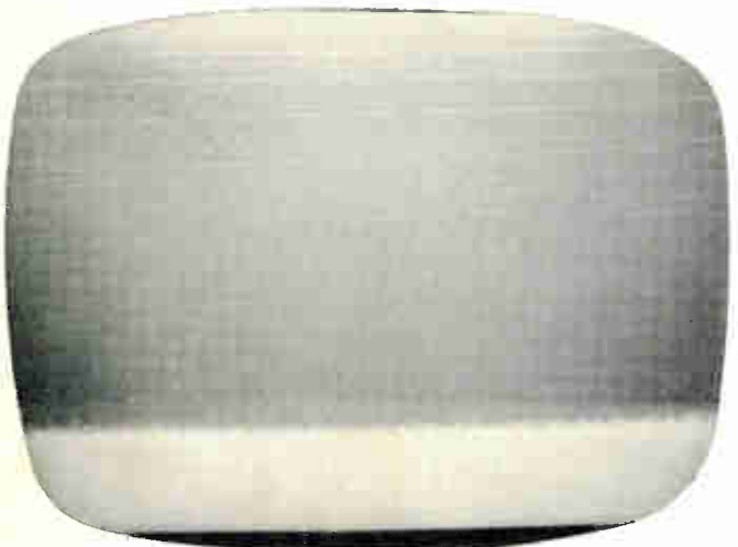
TELE-CLUE M-201: The defect shown was caused by an open AGC capacitor C161 in the "N" chassis between the 12BH7 socket and the 3AU6 1st i-f amplifier socket. A high-level audio buzz was present which varied with the volume control setting. The video and audio defects were due to about 3 volts of 60 cycles a-c which appeared on the AGC line when C161 was open.
