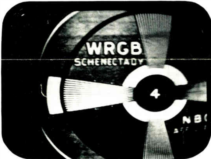
Tele-Clue No. K-75 —This is also the result of a short between cathode and heater in the 6SL7-GT Sync Amplifier and clipper tube and the same explanation as given for Tele-Clue No. 74 will apply here. The only difference is that horizontal synchronization occurs so that the black border can be seen at the left instead of at the right of the picture tube.
