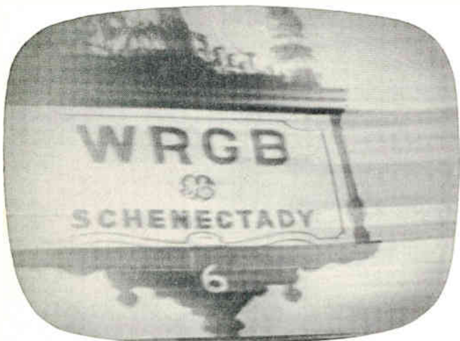
TELE-CLUE F-200: This is another photograph of the same defect shown in Tele-Clue F-199. This shows the streaking in the picture and blanking bar as well as the washed-out appearance at the left side of the picture.
