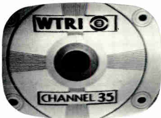
TELE-CLUE O-179. Just about every UHF Converter produced a usable picture from the local station. If a sufficient signal level is present the signal-to-noise ratio of the converter has little importance. The converter used in Tele-Clue O-171 produced the above picture from the local station located about fifteen miles away.
