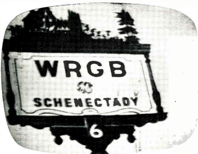
TELE-CLUE E-207 —This shows the effect of "snivets" when a picture is received. A different horizontal output tube may eliminate the "snivets" entirely or change the frequency so the picture is "clean." Another method which may be used is to place an ion-trap magnet over the horizontal output tube as shown in the photographs on the right. The ion-trap is then slowly turned until the "snivets" disappear.
