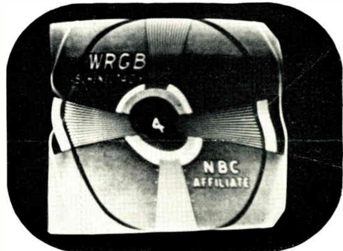
Tele-Clue No. F104. This illustrates another defect due to inadequate filtering. The dark shaded bar is caused by hum in the picture tube grid circuit, while the waviness in the raster edge is the result of hum in the horizontal deflection circuit. This was caused by an open C453 in Figure 2.
