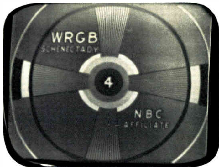
Tele-Clue No. F-111. This photograph illustrates the effect of reducing the line voltage to 110 volts on the same receiver. The height, width, focus and brightness have all been reduced.
