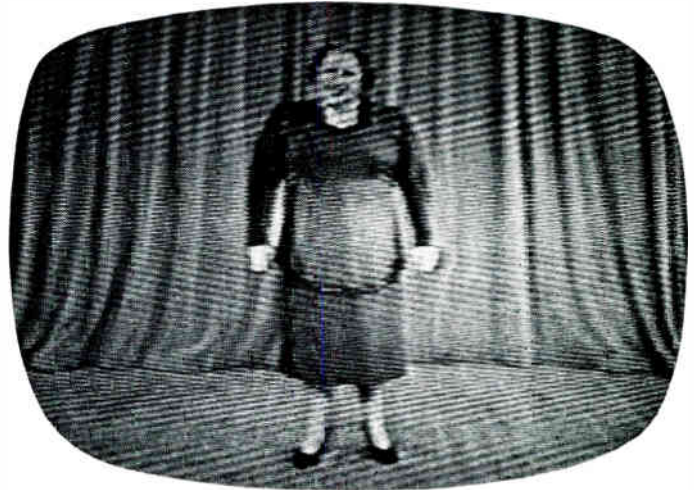
TELE-CLUE J-169: This type of interference may be caused by the oscillator in a UHF converter. It is the result of interaction between the oscillator in the converter and the oscillator in the receiver. In most cases it can be corrected by adjusting the fine-tuning control on the receiver. If this control does not have sufficient range to eliminate the interference, try adjusting the oscillator slug.
