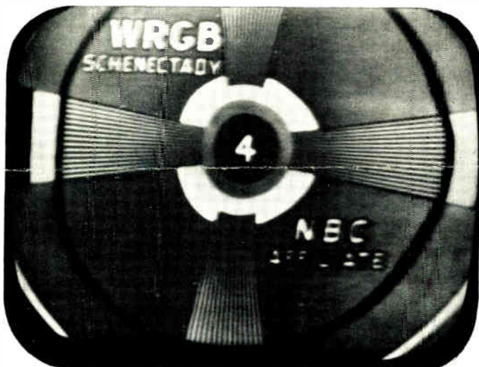
Tele-Clue No. K-107. The above photograph was taken with the contrast control set at minimum (counterclockwise). The defect shown here was due to 50K ohms leakage across C-354 in Fig. 1. Incidentally, if this capacitor is completely shorted, horizontal oscillation is "killed," resulting in complete loss of any illumination on the picture tube. The vertical syncs slightly above normal as can be seen in the above photograph. If C351 is leaky the picture will appear practically the same as the above except that the vertical will sync at the normal point.
