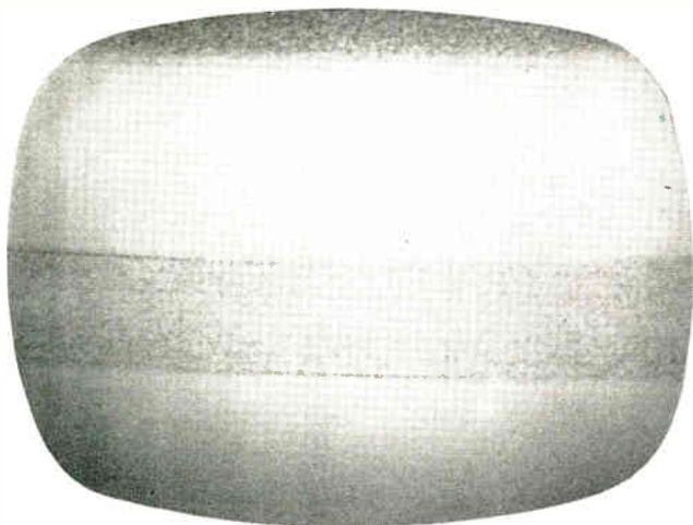
TELE-CLUES F-214 & F-215: The 120-cycle bars seen in Tele-Clues F-214 and F-215 were caused by a gassy 5U4G rectifier tube. These bars could also be seen in the background on some stations, but varied in intensity on different stations.
