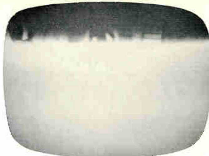
TELE-CLUE M-202: This defect is the same as Tele-Clue M-201 but at a different setting of the vertical hold control.
