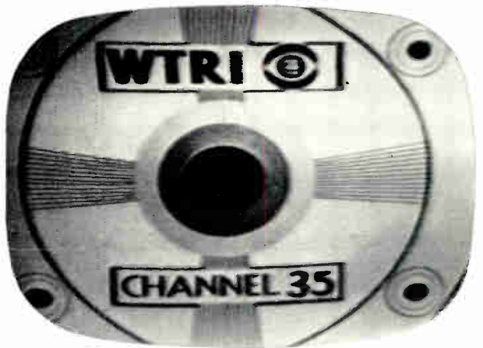
TELE-CLUE O-179. Just about every UHF Converter produced a usable picture from the local station. If a sufficient signal level is present the signal-to-noise ratio of the converter has little importance. The converter used in Tele-Clue O-171 produced the above picture from the local station located about fifteen miles away.
