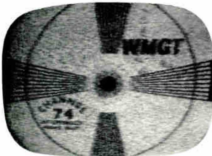
TELE-CLUE O-177. Channel 74 strip in the same receiver (cascode type head-end).
