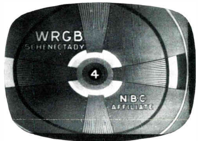
TELE-CLUE E-162. When three quarters of the ferrite core is used most of the picture assumes normal proportions. One portion will however be reduced in size depending on the position of the missing core section. In the above photograph the top right quarter is slightly compressed.
