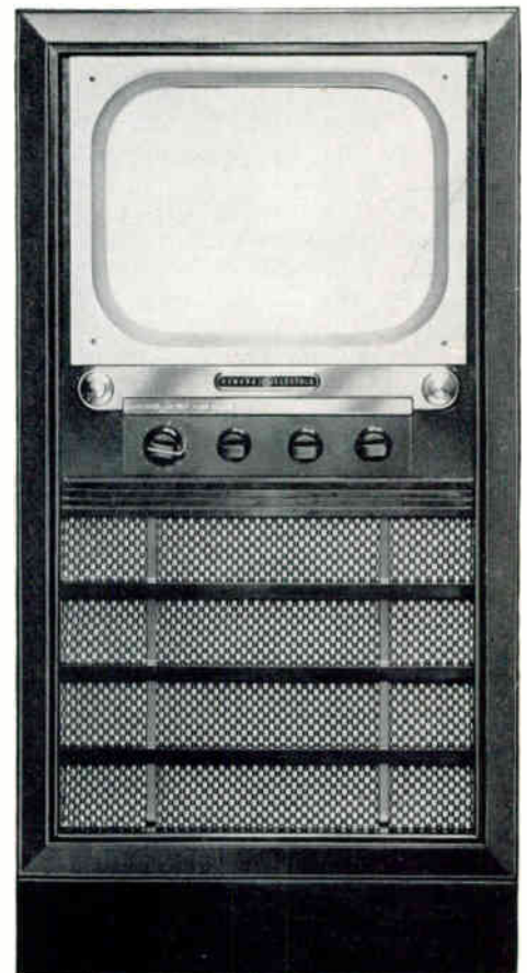
Fig. 2. General Electric Model 10C101 after it has been converted to use a fourteen inch picture tube.
