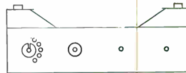
Fig. 3B. The vertical side pieces were bent to support the bottom of the 14CP4 picture tube.
