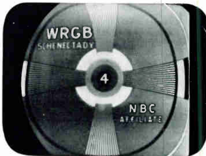
Tele-Clue No. E96. The displacement to the left shows the effect of shorting out the .5 mfd capacitor C 377 in Fig. 2. This condition is the result of additional d-c flowing through the horizontal deflection coils. If this capacitor shorts out it may be impossible to center the picture.
