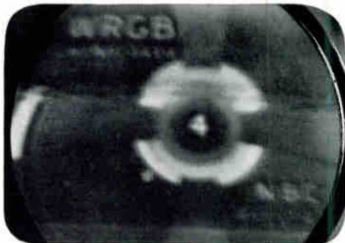
Tele-Clue E94. The increase in horizontal and vertical size as well as the loss in brightness indicates a loss of high voltage. This was caused by a poor connection which developed an arc under the rubber cover at the anode of the picture tube.
