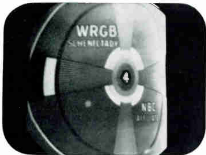
Tele-Clue No. E95. The dim picture with poor horizontal linearity, insufficient width and excessive height was caused by an open in the .5 mfd capacitor C 377 in Fig. 2. This condition is a result of placing a high impedance in series with the horizontal deflection circuit and is caused by an open or very low capacity value of the series capacitor, C 377, to the horizontal deflection coils. This reduces current to the horizontal deflection coils; however, the shunting resistor R 377, passes some current to the coils when capacitor C 377 is open, thus permitting some sweep but with reduced picture tube anode voltage. In some receivers, resistor R 377 will overheat upon opening of capacitor C 377 because of excessive current. High leakage in capacitors C 373 or C 374 will produce similar results except that the linearity will be better.
