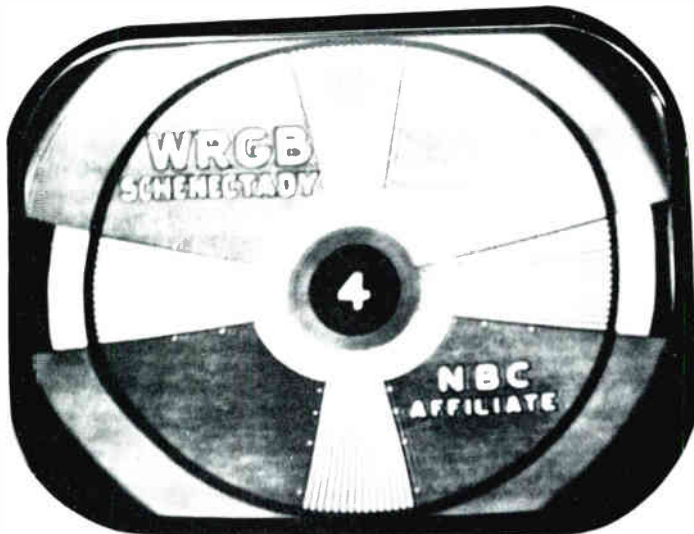
Tele-Clue No. 49—The neck shadows which appear in this photograph are due to a 50° deflection yoke being used on a picture tube which requires a 70° deflection yoke.
