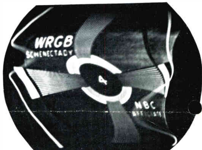
Tele-Clue No. 32 This Tele-Clue is similar to No. 31 except that it indicates the effect of additional a-c hum being present in both the video and sweep circuits. This was due to the total capacitance of C-383 and C-384 in Fig. 3 being reduced to a total of 40 mfd.
