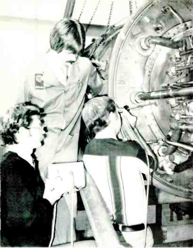
Evendale's Rick Richards (left) watches students inspect an engine's interior using a bore-scope while Jim Broadnax (above) guides a student through engine disassembly. Below: Lynn's Fred McGarry leads classroom discussion on compressor components.
