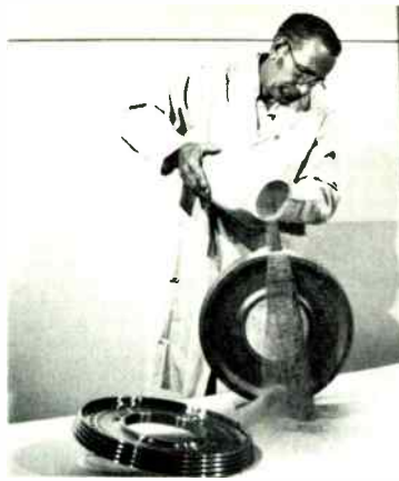
Faced with increases in material costs, Evendale GE is using powdered-metallurgy process to produce many of its aircraft engines.
