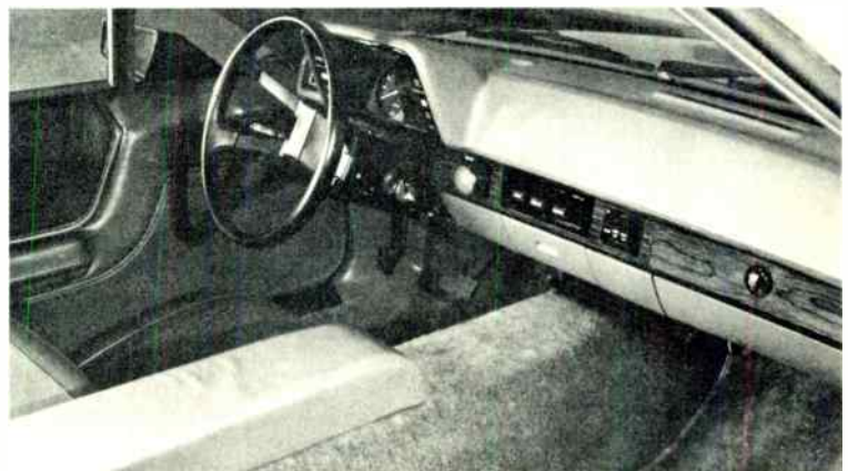
All that’s needed to shift the ETV-1 is a flick of the finger. Three push-buttons, mounted on the dashboard, control the gears.
