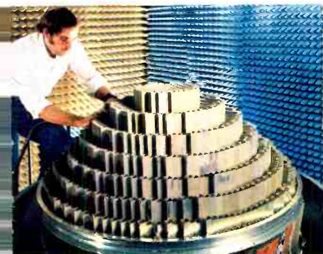
Valley Forge's Microwave Communications Center offers special abilities in high-frequency communications systems. Shown: big wave-guide antenna used in receiving satellite transmissions.
