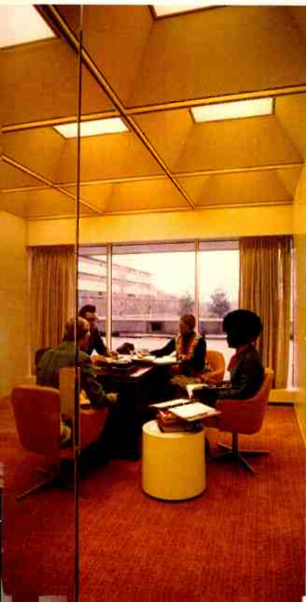
New General Electric Headquarters, well on its way to completion amid meticulously landscaped hillsides with terraced rock walls, already includes finished offices, as previewed at left. Helicopters were used to lower air conditioning units into place on the buildings' rooftops. Integrated modular ceiling units provide heat and air conditioning outlets as well as lighting.
