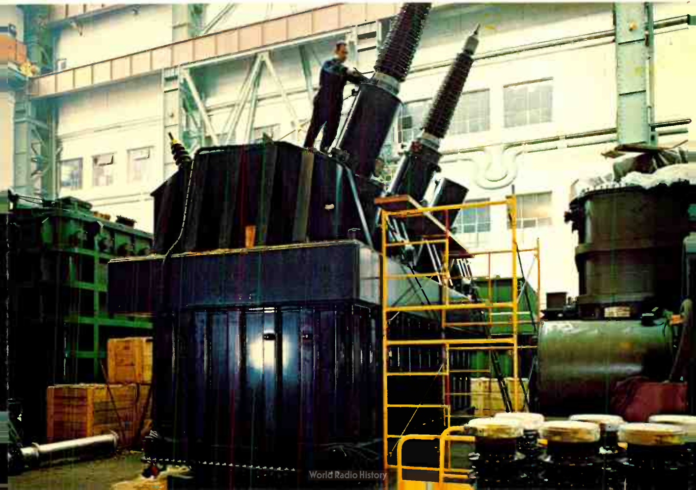
G double E signs along Spanish roadways remind passers-by of General Electric Española, Spain's leading electrical manufacturer. Española is equipped to build large electrical equipment for the Spanish market. Below: 435-MVA transformer in final assembly at Galindo plant in Bilbao.
