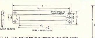
FIG. 12. DIAL ESCUTCHEON is formed ¼-inch thick plastic with window slot for dial scale. It may be painted in a color which matches the color scheme selected for the receiver.
