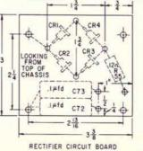
FIG. 13. ASSEMBLY of the rectifier circuit board, looking from top of chassis. Mounting holes in corners should match the mounting bolt locations on the power transformer.
