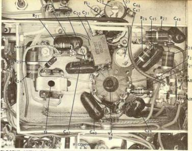
CLOSEUP VIEW OF the 455-kilocycle second IF amplifier (V<sub>4</sub>) compartment. The neutralizing capacitor (C<sub>46</sub>) which assures stable operation is on the 12-pin compactron tube socket. Note the shield partition running across the 9-pin miniature tube socket for  $FL_1$ .
