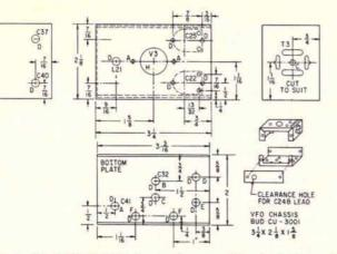
FIG. 4. VFO SUBCHASSIS layout diagram. Holes in bottom plate marked "A" through "F" are for small feedthru bushings (National TPD), and  $C_{32}$  and  $C_{41}$ . They should be drilled through the main chassis to allow connections to be made below the chassis.
