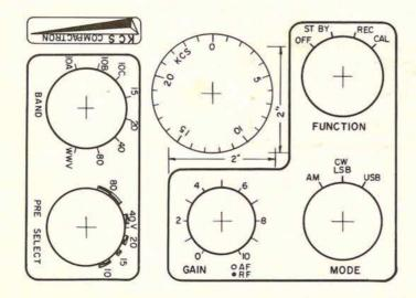
FIG. 16. CONTROL MARKINGS used on the KCS receiver, shown half size. Halmar Electro-Kit name plate process<sup>2</sup> was used to make up marking plates on the model receiver.
