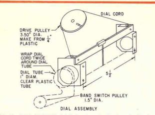
FIG. 11. DIAL ASSEMBLY detail drawing, showing how the brackets, dial scale tubing, runner plate for the pointer, and dial cord and pulleys are assembled. A second dial cord rotates the dial scale, driven from a pulley on the bandswitch shaft between the panel and chassis, as shown in Fig. 8.
