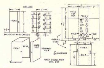
FIG. 5. FORMING AND DRILLING diagrams for the first oscillator coil box which houses  $L_{13}$  to  $L_{20}$  on the chassis of the receiver. Holes for the coils are drilled after folding the main piece. Matching holes for No. 6-32 machine screws are drilled into the main chassis.
