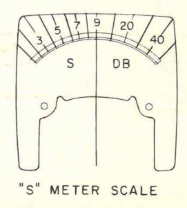
FIG. 15. "S"-METER SCALE, drawn in full size for G-E type DW-91 2½-inch square panel meter.
