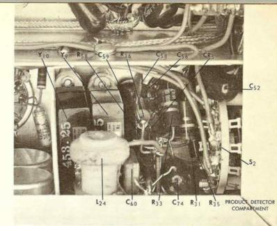
PRODUCT DETECTOR section ( $V_{\theta}$ ) is detailed in this view of the front right-hand corner of the receiver.
