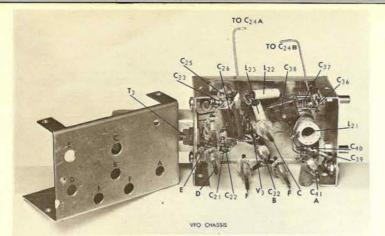
INSIDE VIEW of VFO-second mixer (V<sub>3</sub>) subchassis with bottom cover plate (at left) removed. Machine screws on both sides of first IF transformer (T<sub>3</sub>) are for grounding lugs on inside of box to which grounded ends of  $C_{22}$  and  $C_{25}$  are connected. Note that opening is cut in one side of bottom cover for cover plate which provides access to inside of VFO box after it is installed on chassis of receiver.
