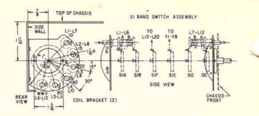
FIG. 8. BANDSWITCH ASSEMBLY, showing the positions of the switch wafers and coils. The brackets on which the RF coils ( $L_1$  to  $L_6$ , and  $L_7$  to  $L_{12}$ ) are mounted are cut as 2%-inch diameter circles from  $V_{16}$ -inch thick sheet aluminum, then drilled, trimmed and bent as shown.
