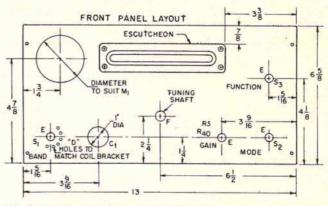
FIG. 7. PANEL LAYOUT diagram for the receiver. Holes for the lower row of controls are drilled through into the front of the chassis, except for the 1-inch diameter hole for the planetary reduction drive on  $C_1$ , which is  $\frac{3}{8}$ -inch diameter in the chassis. The circle of holes surrounding the bandswitch shaft are drilled using the coil bracket shown in Fig. 8 as a template.
