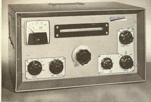
NEATNESS AND SIMPLICITY of front panel of the receiver is apparent in this view. Vernier scale on tuning knob has 100 divisions, but scale showing 25-kilocycle-per-knob-turn tuning rate can be applied over it. Concentric type potentiometers are used on RF and AF gain controls. "S" meter is standard General Electric DW-91 "Big Look" meter with hand-calibrated scale added by W7KCS/9.
