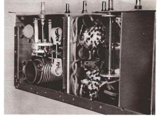
EXCITER COMPARTMENTS in the r.f. unit. Plug-in coils have been removed to show the coil sockets mounted on metal pillars ¾ of an inch high. All partitions and shelves were fabricated from 1/16-inch thick soft sheet aluminum. The crystal sockets were mounted on a bracket drilled to match the socket holes.
