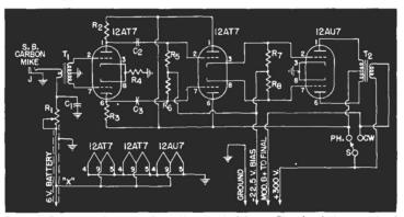
Fig. 9. Schematic diagram of the Mobile Modulator. The 6-volt battery lead should be of heavy shielded wire, with a switch to turn off heater power.
