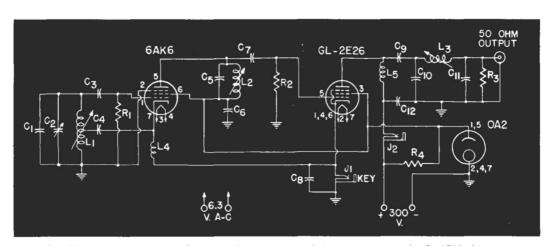
Fig. 3. Schematic diagram of the Emergency-Portable Rig. Jack J2 is for measuring the GL-2E26 plate current.
