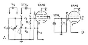
Fig. 4. Alternate oscillator grid circuits for (A) both crystal controlled and VFO operation, and (B) crystal controlled operation only, eliminating  $C_1$ ,  $C_2$ ,  $C_3$ ,  $C_4$ ,  $L_1$  and  $L_4$ .
