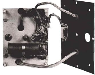
Fig. 10. Layout and construction details of the Mobile Modulator. The 12AT7 voltage amplifier is the shielded tube at the bottom next to the microphone transformer, T<sub>1</sub>.
