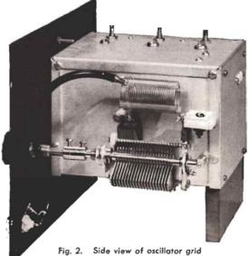
Fig. 2. Side view of oscillator grid tank circuit box showing C<sub>13</sub>, C<sub>14</sub>, C<sub>15</sub>, L<sub>4</sub> attached to removable cover. A coupling coil,  $L_5$ , feeds the output through  $J_4$  when a longer cable is desired.
