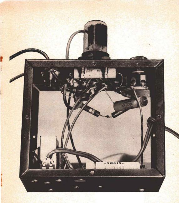
signal generator, an RF voltage of 4 volts read 3.8 volts with the Adapter-multi-meter combination. Above 10 megacycles the sensitivity fell off and the Adapter no longer gave an accurate reading. However, the presence of RF on the coil of a grid dip oscillator was still indicated by the Adapter up to 250 megacycles.
