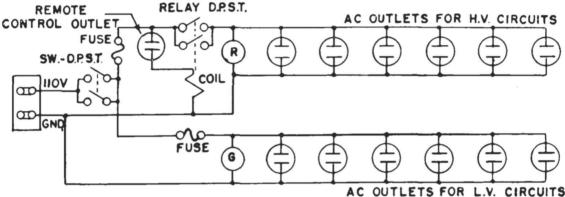
The circuit is simple and provides for remote control via the a-c type female outlet on the front of the panel. On the rear of the unit are two rows of a-c outletsboth supplying 110-volt a-c. The bottom row of six outlets is controlled by the front panel switch and is used for filament circuits in other pieces of equipment. The top row of outlets is controlled by the same switch plus the relay, and offers 110-volt a-c for the highvoltage plate transformers of various pieces of equipment.
