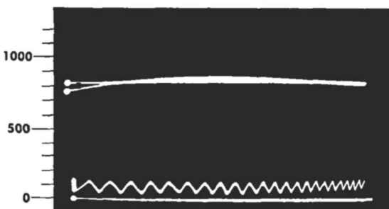
FIG. 8 Load removed ( C_a=0; C_b=90 mfd)
