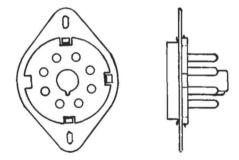
A few notes: Amphenol sometimes supplies a thicker mounting plate. Only the thinner ones can be used here. They seem to be the commonest kind. Also, a vise or pair of pliers can be used gently to push the base into the plate. It is a good snug fit.
