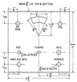
Fig. 7. Front panel layout of Mobile-Marine Receiver.
