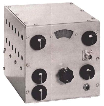
Fig. 1. Front view of the Mobile-Marine Receiver.
