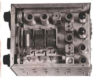
Fig. 4. Top view of the Mobile-Marine Receiver.
