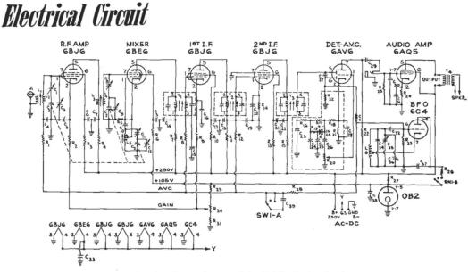
Fig. 2. Circuit diagram of the Mobile-Marine Receiver.
