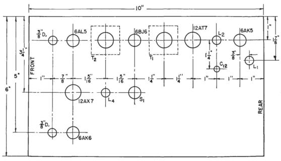
Fig. 5. Chassis layout of 6-Meter CD Receiver
