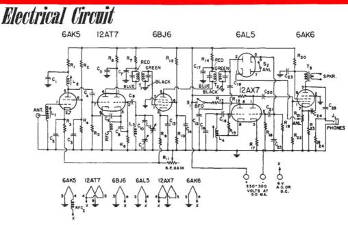
Fig. 2. Circuit Diagram of the 6-Meter CD Receiver
