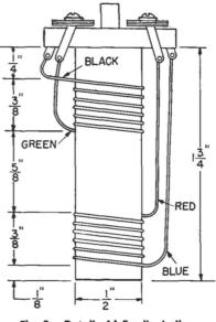
Fig. 8. Detail of I-F coil winding
