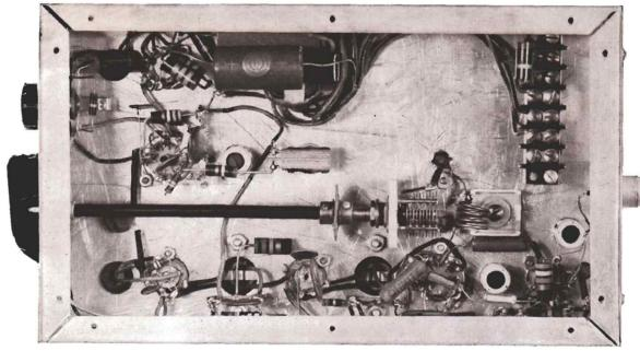
Fig. 3. Underchassis view of the 6-Meter CD Receiver
