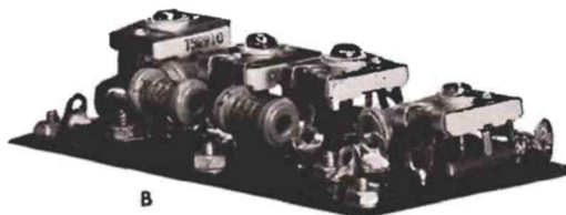
Fig. 3. (A) Mechanical arrangement of the audio phase-shift network. (B) Detail view of the audio phase-shift network
