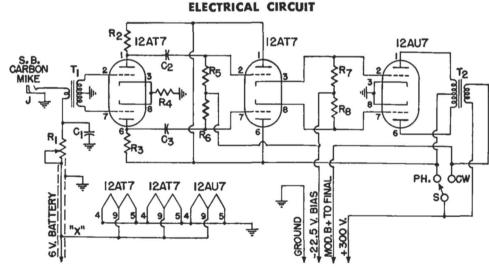
Fig. 2. Circuit diagram of the Mobile Modulator.
