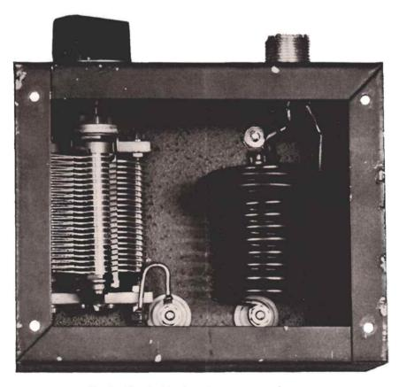
Fig. 6. View looking into the antenna coupler.
