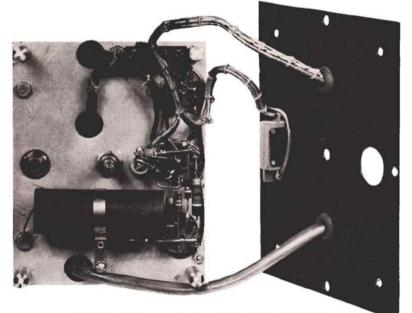
Fig. 3. Under-chassis view of the Mobile Modulator.
