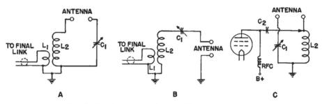
Fig. 7. Circuit diagrams of the mobile and emergency antenna.
