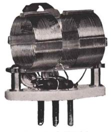
Fig. 7. Detail of Grid Coil
