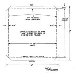
Fig. 11. Detail of Side Shields
