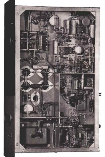
Fig. 6. Under-chassis View of SSB Adapter. Note the Shield Around the Four Tubes on the lower Right Side
