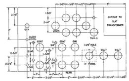
Fig. 7. Layout Guide for SSB Adapter
