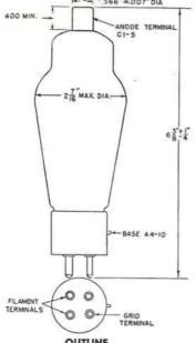
The FG-17 thyratron is a negative-control mercuryvapor tube for use where it is desired to actuate the tube with a change in negative grid voltage. It requires relatively little grid power and is suitable for use in relay circuits where current flow is desired in the absence of grid excitation.
