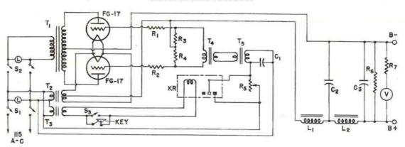
Fig. 1—Circuit Diagram of Power Supply Using Two FG-17 Thyratrons.
