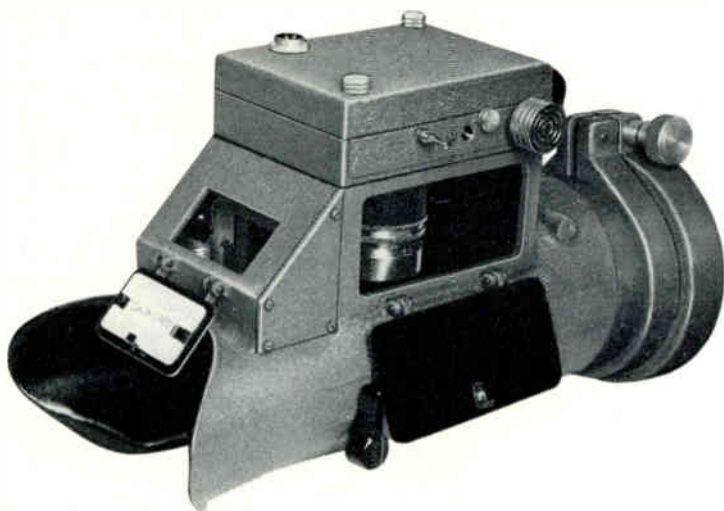
Figure 7. Type 295, with access port open, permitting adjustments of aperture setting. Data card, over viewing port, provides convenient means for recording pertinent information directly on oscillogram. Knob below access port controls mask to close viewing port when in use. Over access port are, from right to left, film-advance knob, frame-counter re-set knob, frame counter, and shutter release.
