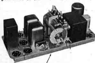
Arrows on the above photograph show some of the cadmium plated parts on Crosley Gembox, Model 608.
