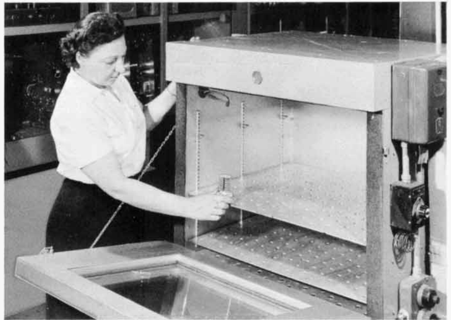
Figure 2. Varnishing and Baking the Coil Form.
