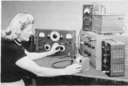
Figure 3. RF Comparison of 245-B RF Voltage Standard to Bolometer Bridge.
