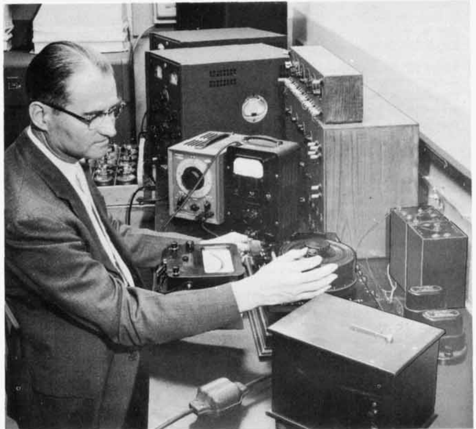
Figure 1. Adjustment of Basic Voltage Standardization Equipment by the Author. Normalized Atmospheric Conditions (Temperature and Relative Humidity) for Improved Stability are Maintained by Air-conditioning Equipment in Background.
