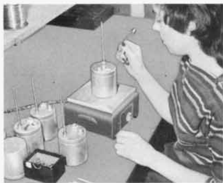
Figure 3. Sealing Operation of Q Standard..
