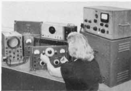
Figure 4. Measurement of FM Deviation and FM Distortion of Type 202-E FM-AM Signal Generator by Use of FM Linear Detector and Associated Apparatus.
