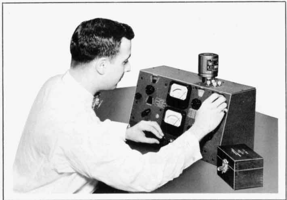
Figure 1. The importance of the quantity Q in the analysis of electronic circuits and components has made the Q Meter a familiar laboratory tool. Here, H. J. Lang, BRC Sales Engineer, is checking the accuracy of a Q Meter Type 260-A with the new Q-Standard.
