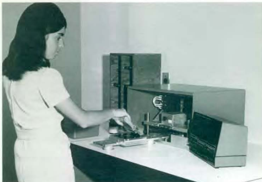
The electrolyte is applied through a template that limits the spread of the gel to the anodizing area.
