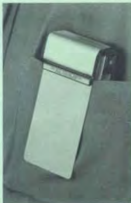
The 1944 Noise-Exposure Monitor
