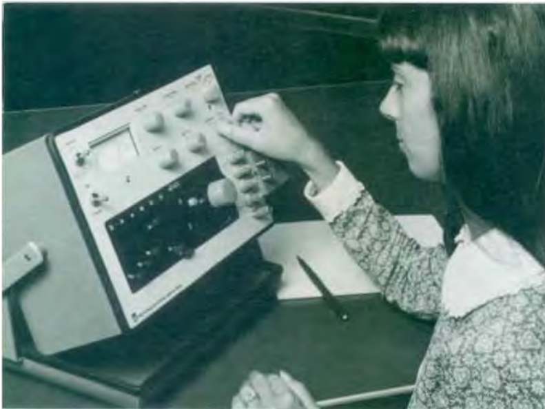
The 1666 is a new kind of low-cost manual bridge with extremely wide range and 0.01% basic accuracy.
