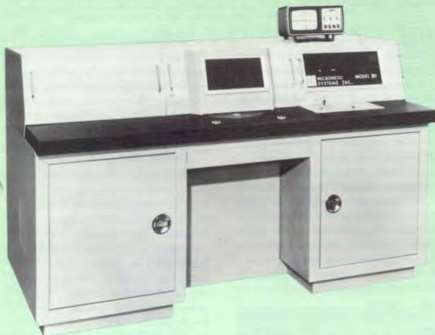
Micronetic's Model 80 Laser-Trim System, being used in telephone tone-generator production.
