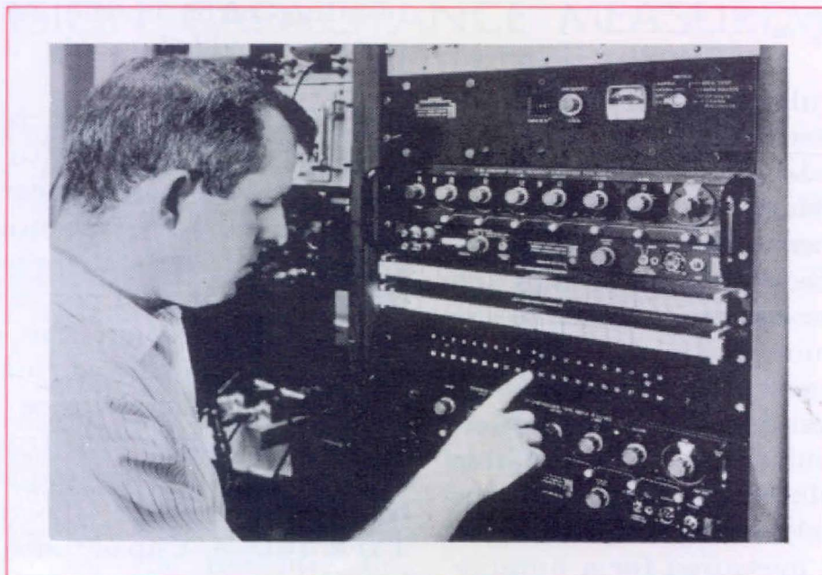
Figure 1. Type 1163 synthesizer under control of 40-channel program unit. Additional frequencies are available in second 40-channel unit.
