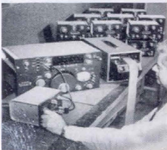
Type 1151-AP Counter measures period of output signal from a Type 1311-A Audio Oscillator. A Type 1137-A Data Printer provides a permanent record.
