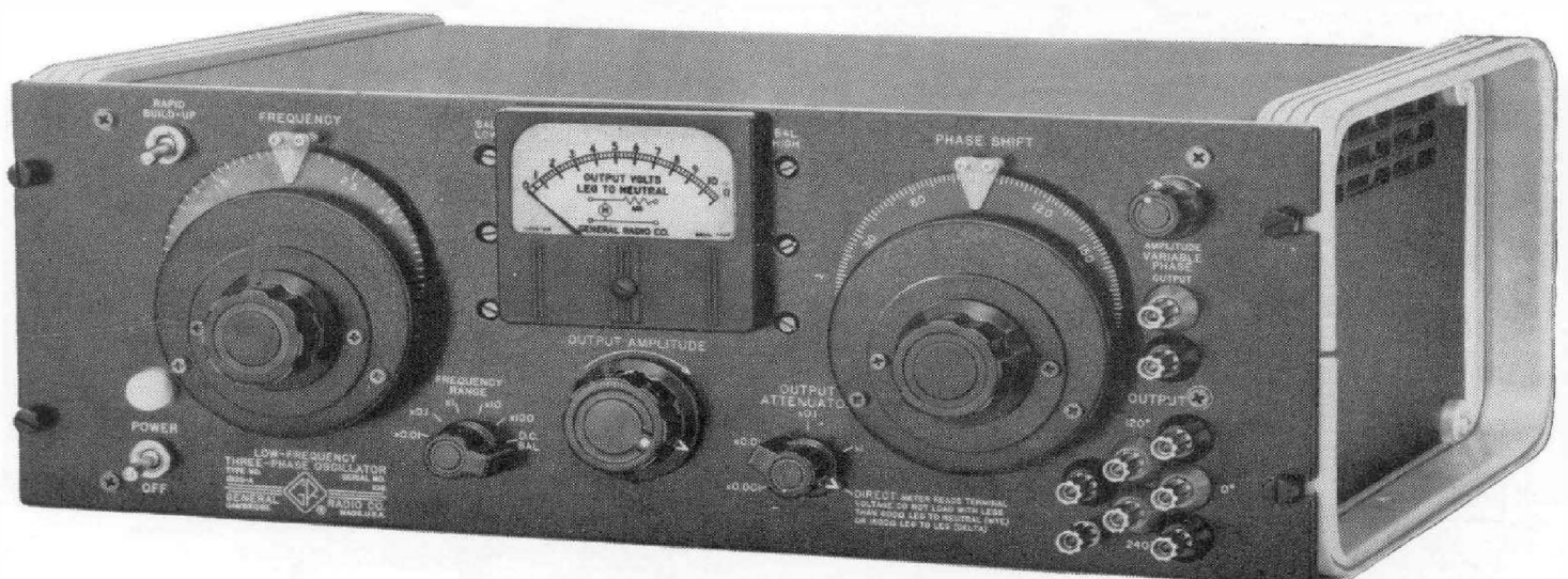
Figure 1. Panel view of the Type 1305-A Low-Frequency Three-Phase Oscillator.
