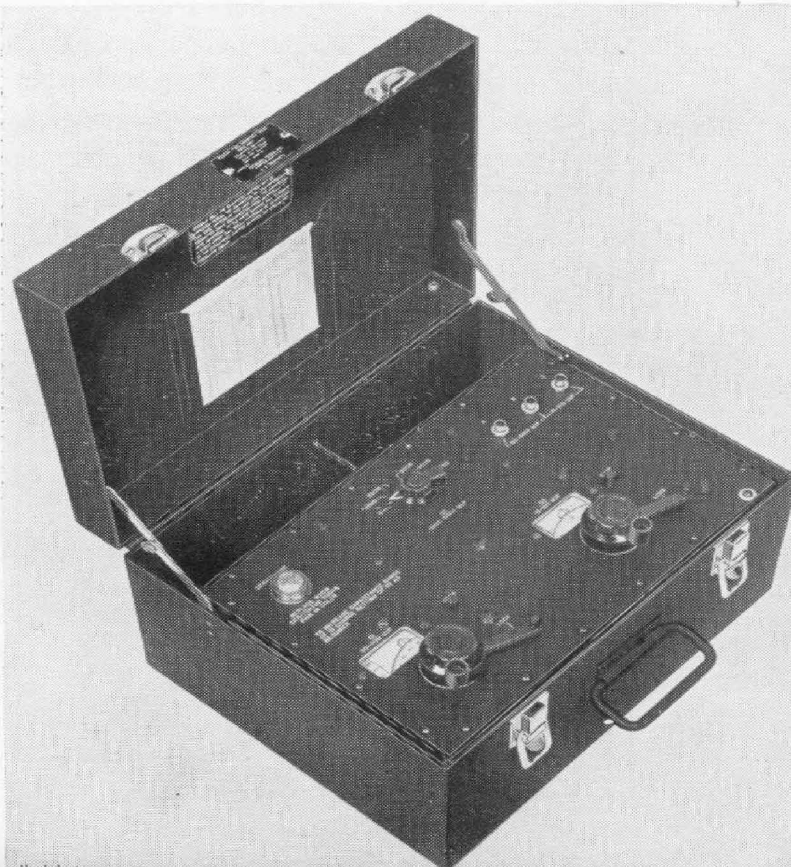
Figure 1. View of the Type P-579 Field Variable Capacitance Tester, mounted in its transit case.
